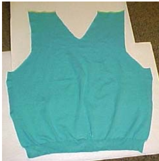
Front panel is shaped and has a finished (contoured) neckline and armholes.
